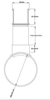
Grates longer than 1500mm supplied in sections. Tile Inserts longer than 1200mm supplied in sections. Channels over 3000mm supplied in sections with joiner. +/-2mm tolerance on dimensions
