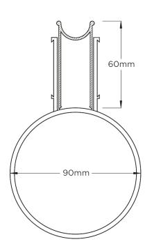
Grates longer than 1500mm supplied in sections. Tile Inserts longer than 1200mm supplied in sections. Channels over 3000mm supplied in sections with joiner. +/-2mm tolerance on dimensions.
