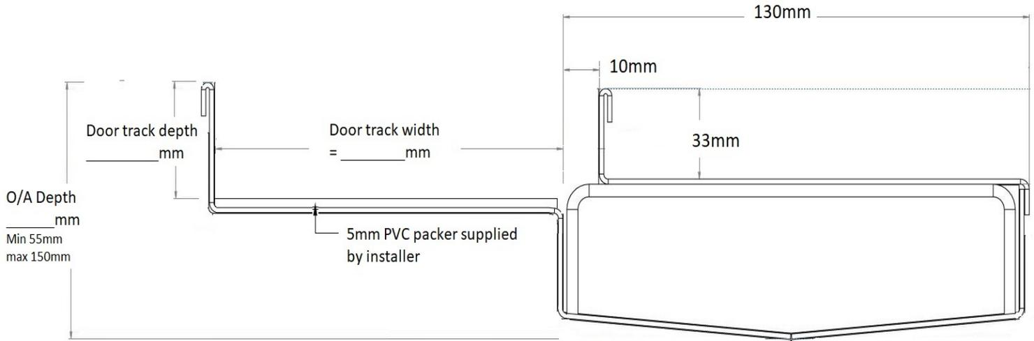
SQ100Ti33DN80 floor wastes to sit above each outlet. Floor waste suits up to a 25mm tile/ stone.
