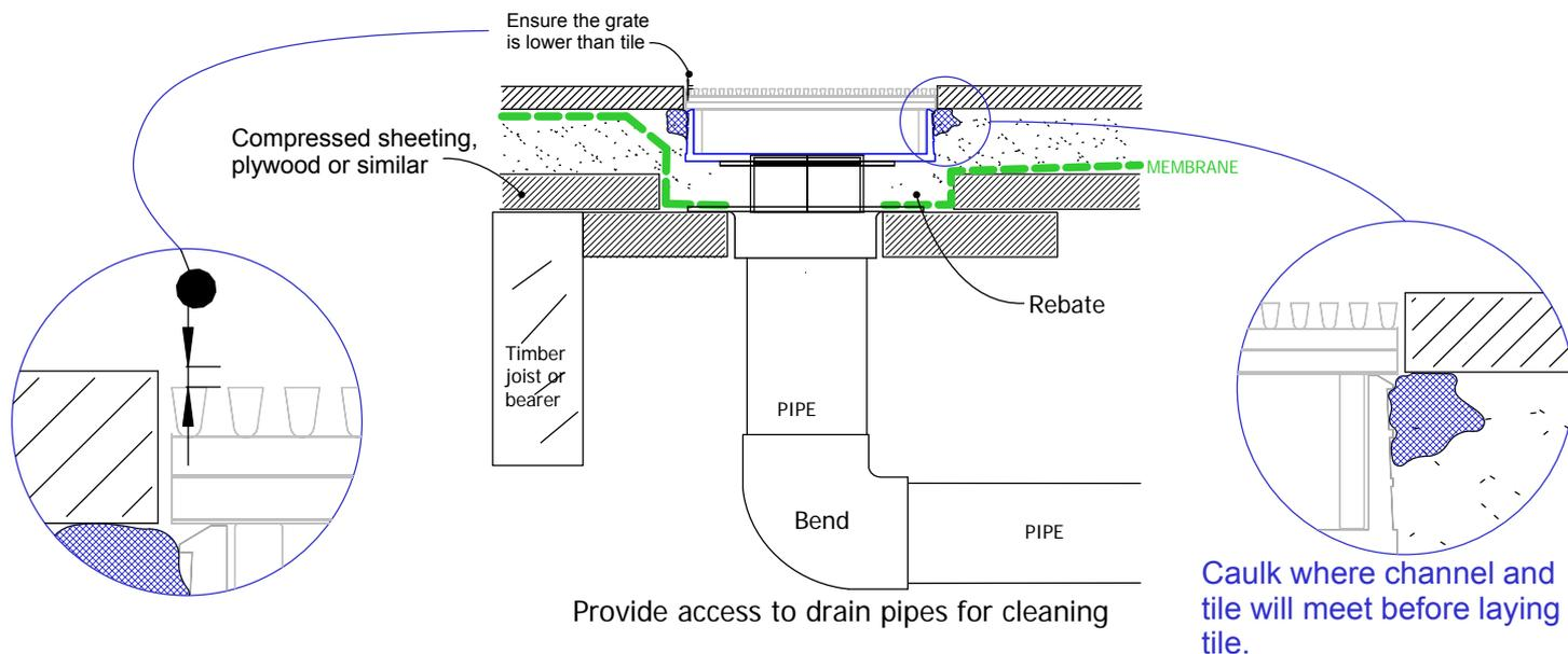
When 100ARG30 is running perpendicular to joist/bearer
