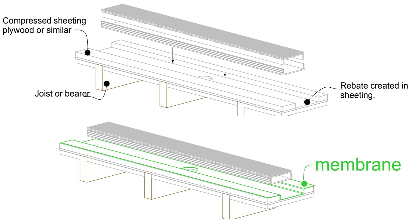
**NOTE: For exterior application allow for expansion of 1mm per metre by using quality suitable flexible sealant on channel joins. Use PVC solvent cement and primer on ends and outlets.**
