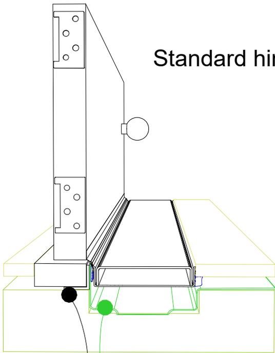
Aluminium angle to support waterproofing and junction between channel and door sil.
