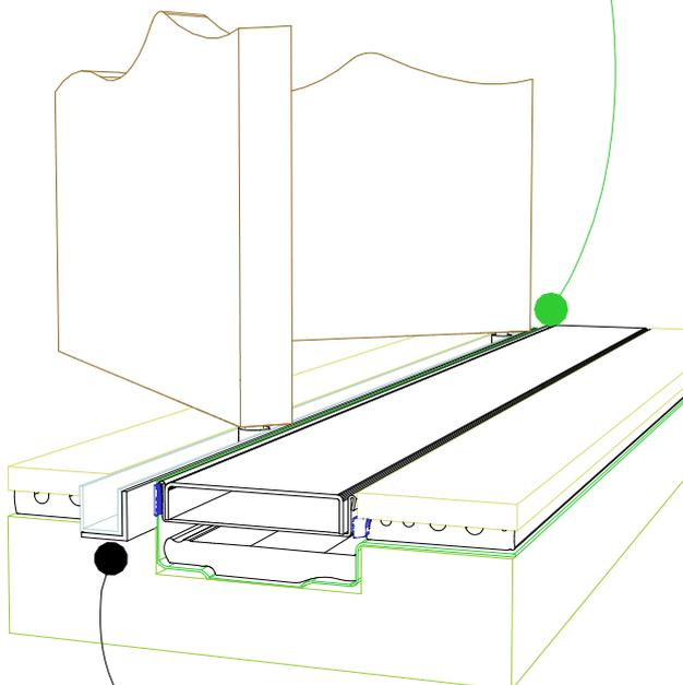
Aluminium angle to support waterproofing and junction between channel and door track.
